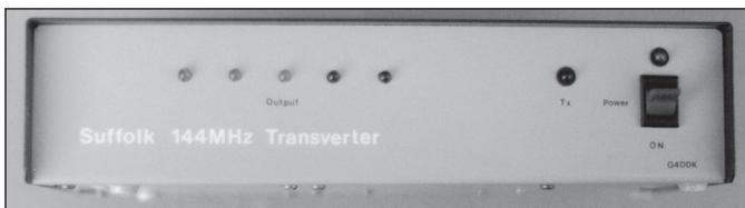
Fig. 8.7. Front panel of the Suffolk transverter
