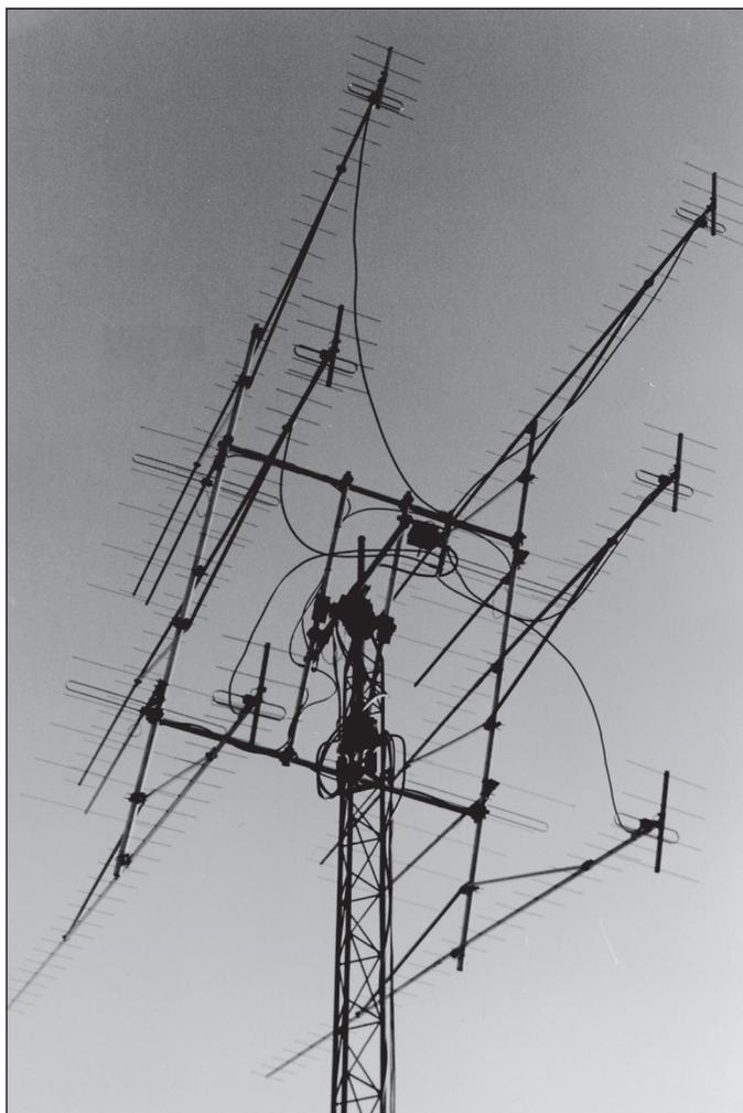
Fig. 7.6. Photo of the six-yagi 432MHz array at DL6WU, with four short 144MHz Yagis stacked between
