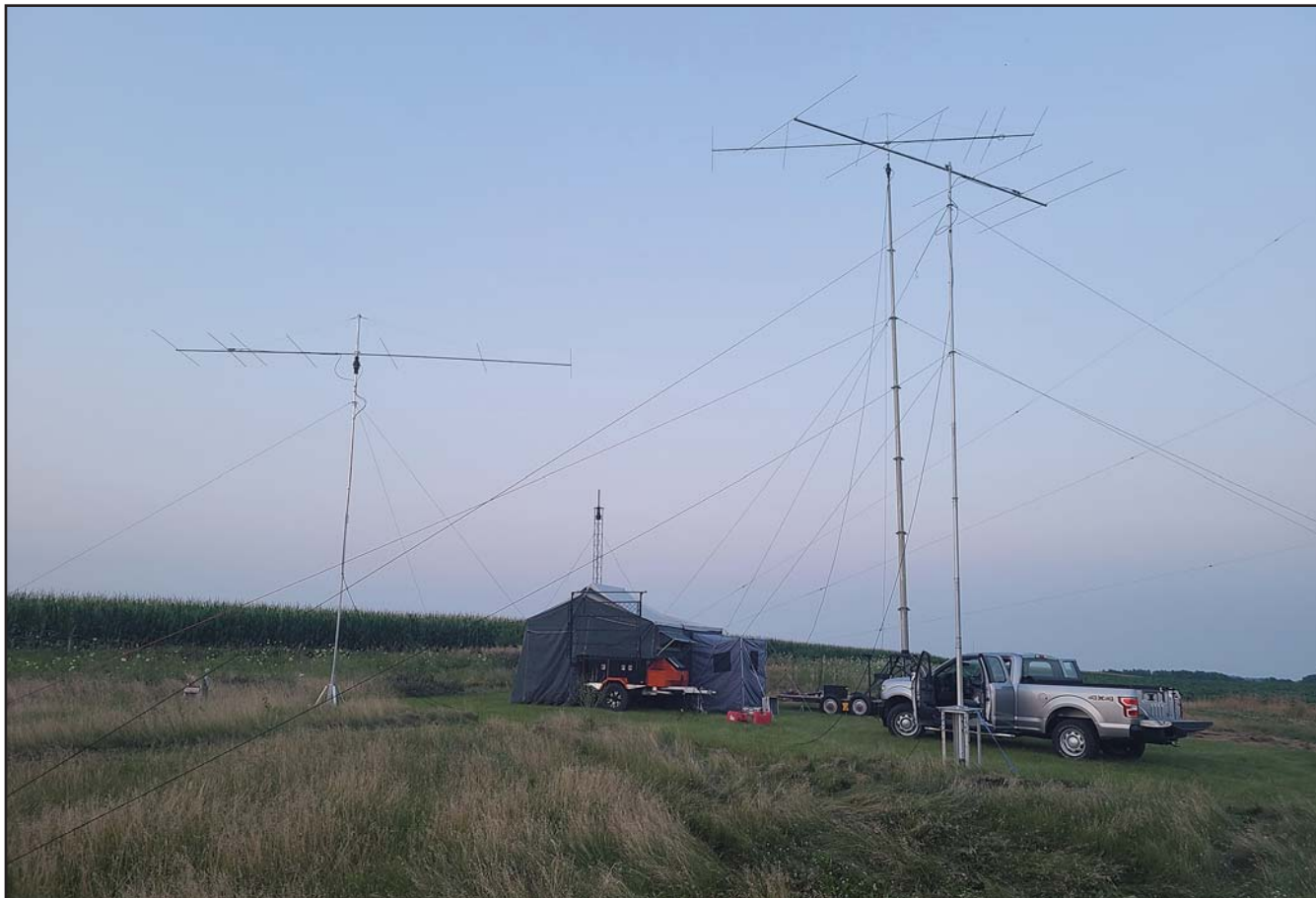
ACØRA's three 6-meter antennas, two 7-element Yagis and a 5-element Yagi, not to mention a 60-foot pneumatic mast for one of the 7-element Yagis. (Photo by ACØRA)
