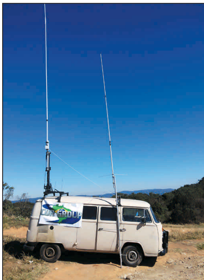
PY2LCD's station at 1130 meters above sea level. The antennas are VictorCharlie0680 for 6 meters (on the left) and a Comet GP9 for 2 meters. The rig was a Yaesu FT-817 powered by a 400-watt wind generator and two batteries.
